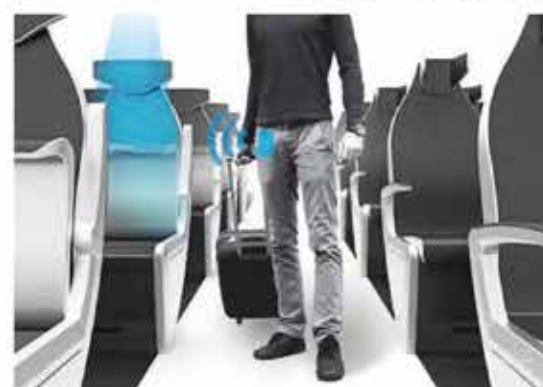
FIGURE 4 (BELOW): AS THE TICKET HOLDER GETS CLOSER TO THE SEAT, THE LIGHT BECOMES BRIGHTER (DESIGN: S AKKERMAN)
